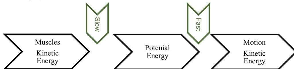
The chemical energy stored in food is transformed into chemical energy in the attacker's muscles, which is transformed into the kinetic energy to cock the siege machine. The energy in the cocked position has now been transformed into potential energy.
