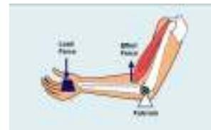
The human arm and an arm in a trebuchet or catapult both act as simple machine levers that can provide a mechanical advantage.
