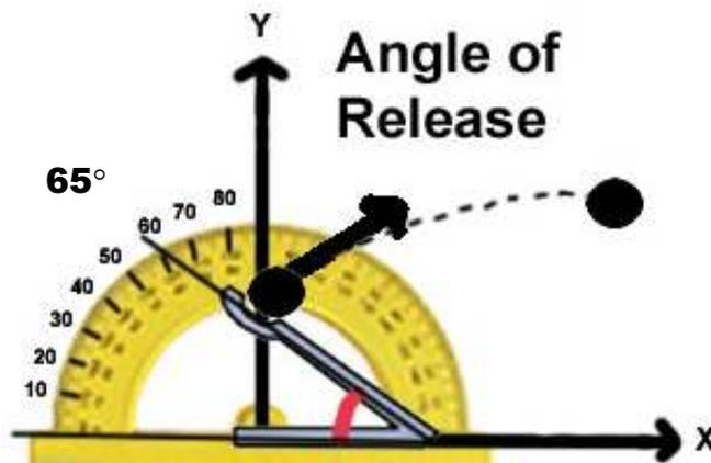
The angle of release can be measured with a **protractor**.
