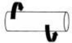
One of the ways that a force can be applied to elastic material in a catapult in order to store potential energy. In ancient catapults torsion was obtained by twisting rope. In the inventor center you may want to twist a rubber band.
