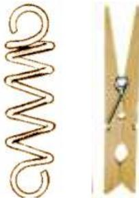
Some kinds of clothespins contain a spring that is holding two levers together at the fulcrum. It takes force to squeeze the two long ends of the lever together because this is changing the shape of the spring. If a clothespin was built into a catapult that potential energy could be released as kinetic energy of motion of a projectile when the pressure is released.
