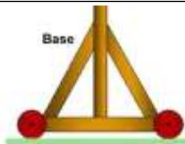
For a catapult or trebuchet to work efficiently it is important for the base to be stable so that when the stored potential energy is released, only the arm and the projectile move, not the base.
