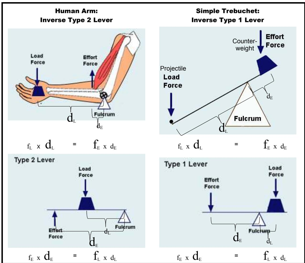
Work is equal to force times distance. The work put in on the effort side of the arm is always equal to the work done on the load side of the arm.
